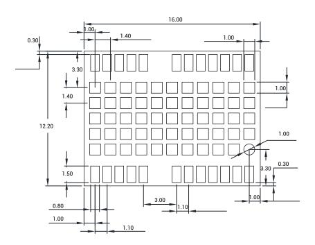
Figure 3-4 Recommended Footprint (Unit: mm)
