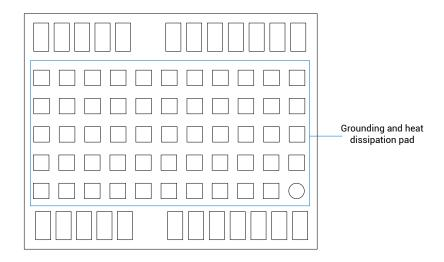
Figure 3-3 Grounding and Heat Dissipation Pads (Bottom View)
