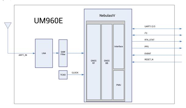
Figure 1-2 UM960E Block Diagram
