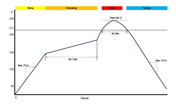
Figure 4-1 Soldering Temperature (Lead-Free)
