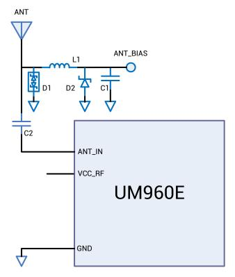
Figure 3-2 UM960E Reference Design for Antenna Bias
